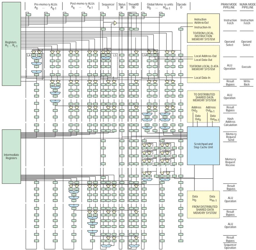
Fig. 4. Block diagram of the MBTAC processor
