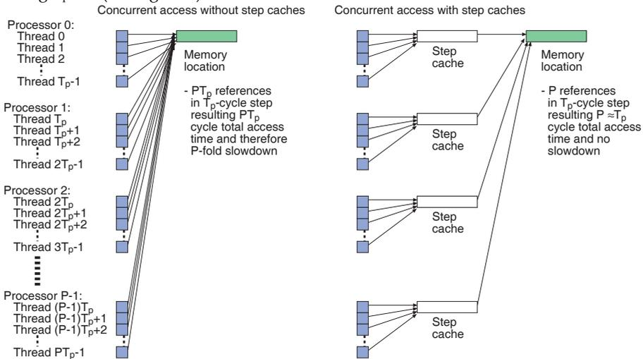
Fig. 6. Step caches for implementing concurrent memory access.
