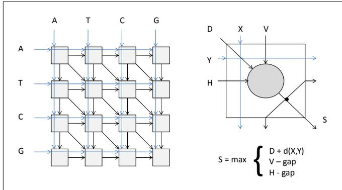
Fig. 5. Implementation of the programming dynamic algorithm on a 2D systolic array. Each cell performs a maximum of three terms. The similarity score is obtained on the bottom right cell in  $2n-1$  cycles ( $n$  is the length of the sequences).
